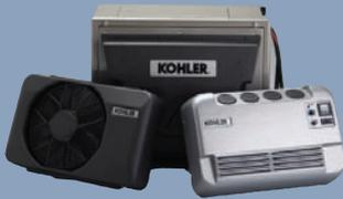
The KOHLER 3APU-HC comes equipped with separate space-saving evaporator and condenser components. It provides an air-conditioning capacity of 12,000 BTU/hour and 10,000 BTU/hour of heating, independent of the truck's climate control system.
